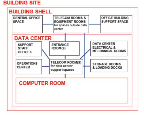
Figure 1. Basic needs diagram of your owned datacenters [16]
