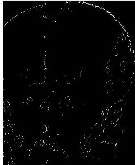
Figure 11. Crack map after interpolation
