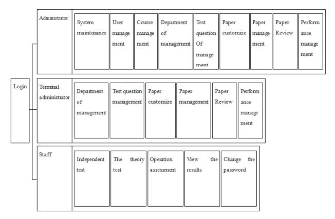
Figure 1. The function structure of the assessment system
