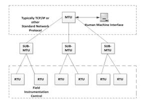
Figure 1. Components of a SCADA System
