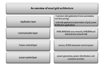
Figure 2. An overview of the smart grid architecture
