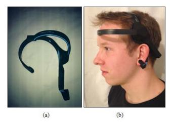
**Figure 1.** NeuroSky MindWave device: (a) Appearance of the device; (b) Example of mounting the device on the head of the tester
